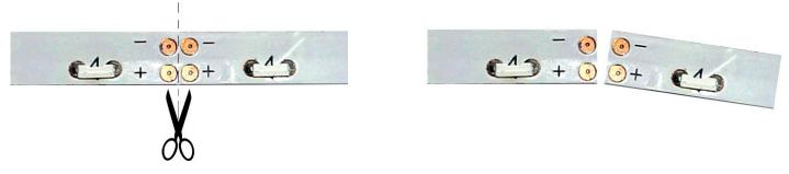
Cut the Strip along the line with the 2 solder pads on either side of the cut.
